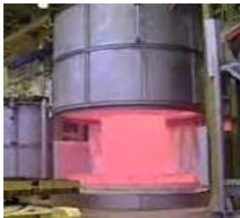
BELL TYPE FURNACE
